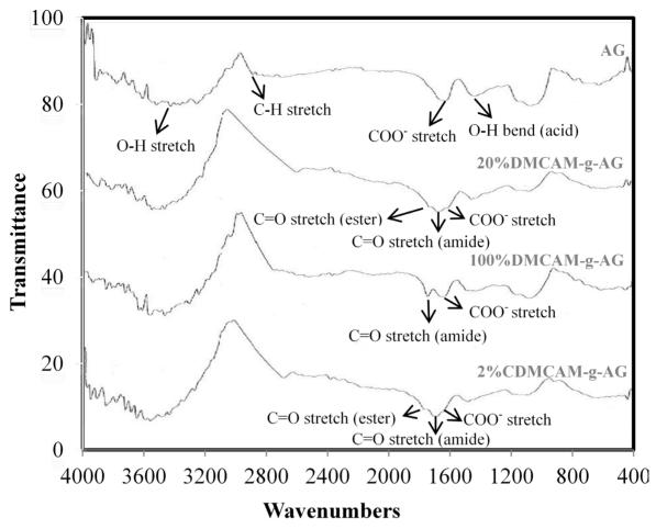
Figure 1. FT-IR spectra of AG and representative graft copolymers (20%DMCAM-g-AG, 100%DMCAM-g-AG and 2%CDMCAM-g-AG).
