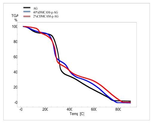
Figure 2. TGA curves AG and the respective graft copolymers.
