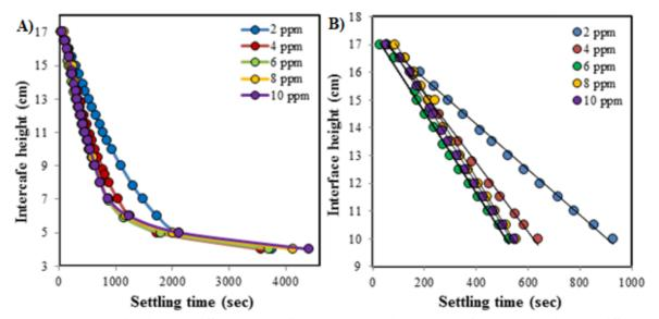
Figure 4. A) Suspension line descent at different dosages of 40%DMCAM-g-AG B) Linear region of suspension line descent at different dosages of 40%DMCAM-g-AG.
