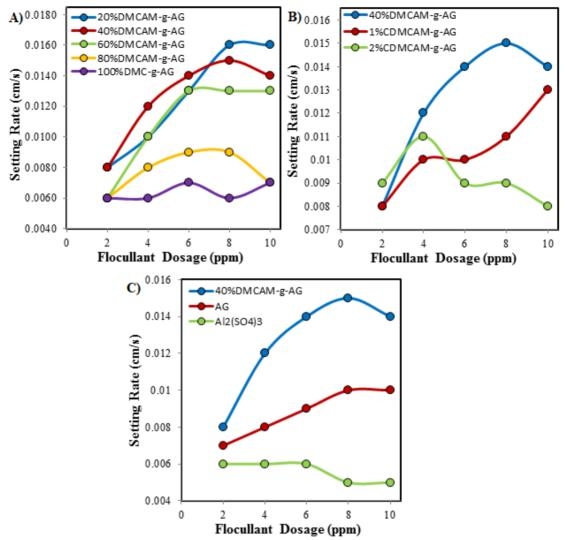
**Figure 5.** A) Flocculation characteristics of AGs grafted with polyacrylamides in different cationic ratios B) Effect of crosslinking on flocculation properties C) Flocculation characteristics of AG, 40%DMCAM-g-AG and  $Al_2(SO_4)_3$ .
