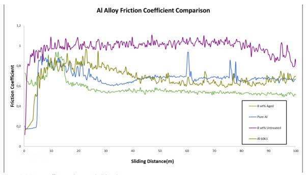
Figure 5. Friction coefficients change with sliding distance.
