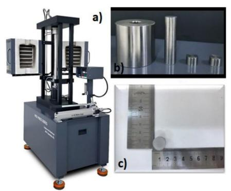
Figure 2. a. Hot pressing machine b. Die and punches made of hot work tool steel c. an example of produced samples
