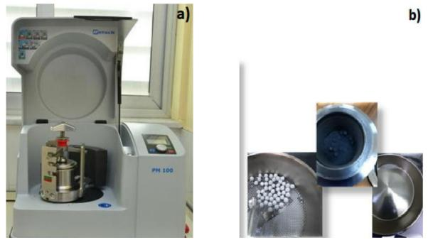
Figure 1. a. Ball milling machine b. Stainless Steel jars and zirconia balls with 10 mm diameter
