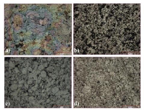
Figure 7. Microstructures of the specimens. a. Pure Al untreated b. Al6061 without reinforcement and heat treatment c. Al6061 8 wt% GNP untreated d. Al6061 8 wt% GNP and artificially aged.
