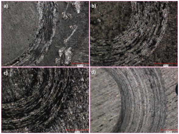
Figure 6. Wear surfaces of the specimens a. Pure Al untreated b. Al6061 without reinforcement and heat treatment c. Al6061 8 wt% GNP untreated d. Al6061 8 wt% GNP and artificially aged
