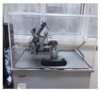
Figure 4. CSM Tribometer.
