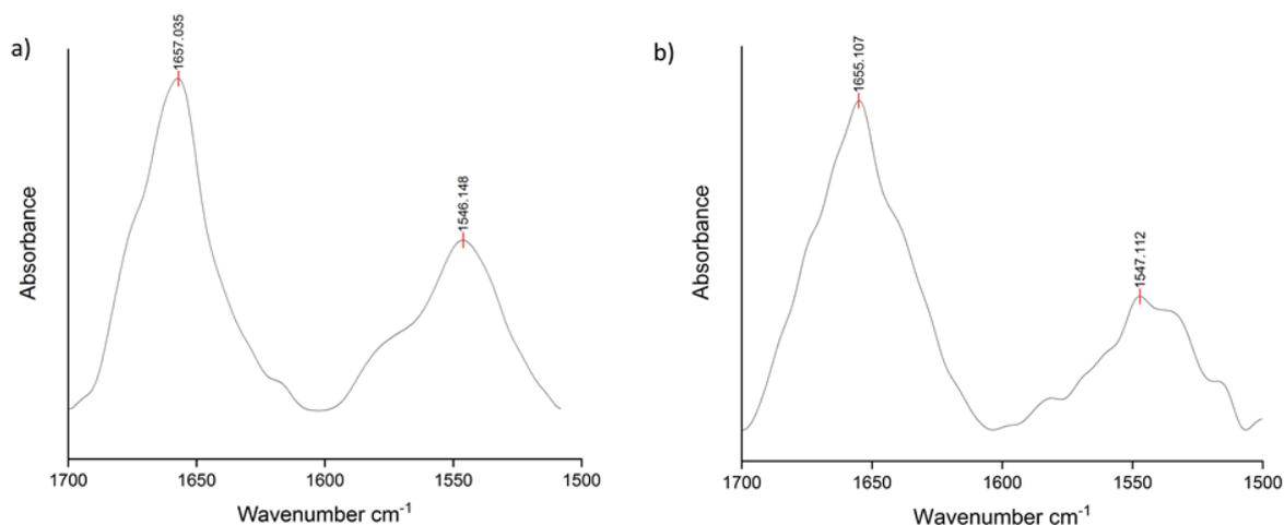
**Figure 4.** Amide-I and II bands of BSA adsorbed on a) PHB and b) PHBV.
