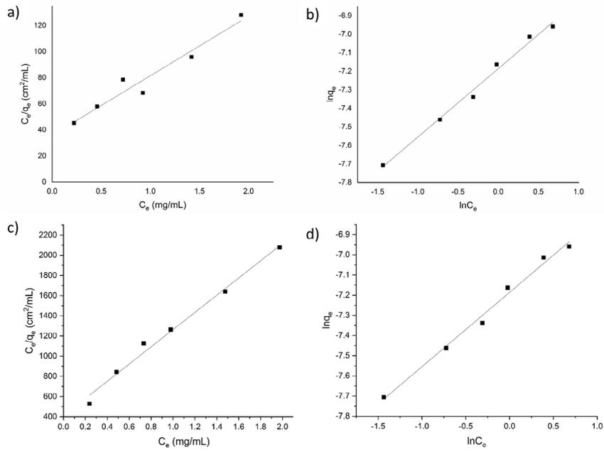
**Figure 2.** a) Langmuir and b) Freundlich fitting curves of BSA adsorption on PHB and c) Langmuir and d) Freundlich fitting curves of BSA adsorption on PHBV.
