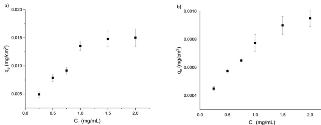
**Figure 1.** The adsorption isotherms of BSA on a) PHB and b) PHBV.
