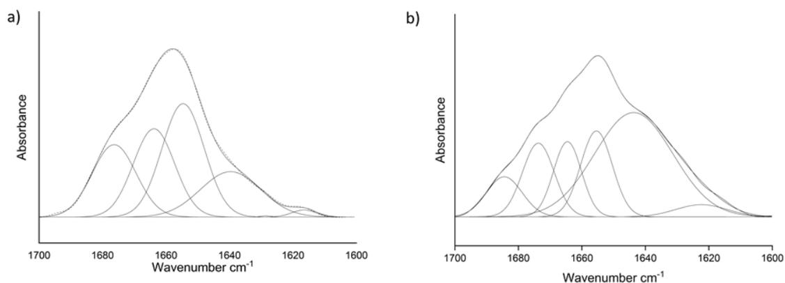
**Figure 5.** Deconvolution of the amide-I band of BSA on a) PHB and b) PHBV.
