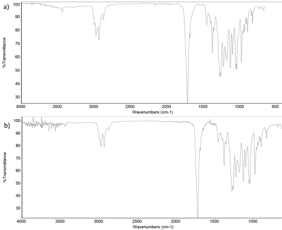
**Figure 3.** FTIR-ATR spectra of a) PHB and b) PHBV. BSA adsorption on PHBV.
