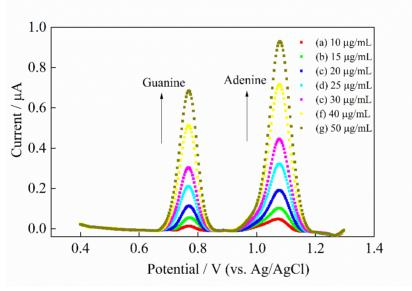
**Figure 4.** DPVs of the oxidation peaks of the guanine and adenine at the dsDNA concentrations varying from 10 to 50  $\mu$ g/mL in ABS (pH 4.8) at the GCE/ERGO/P(PDCA).
