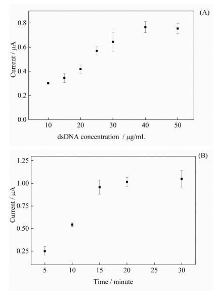
**Figure 5.** DPVs of the oxidation peaks of the guanine and adenine at the dsDNA concentrations varying from 10 to 50  $\mu$ g/mL in ABS (pH 4.8) at the GCE/ERGO/P(PDCA).
