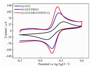
Figure 3. Cyclic voltammogram of (a) GCE, (b) GCE/ERGO, (c) GCE/ERGO/P(PDCA) in 0.1 M KCl solution containing 5.0 mM  $Fe(CN)_6^{3/4}$ .
