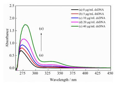
Figure 8. UV-vis spectra of HDN (65.6  $\mu$ M) in the absence and presence of dsDNA in the range of 5.0 40.0  $\mu$ g/mL.
