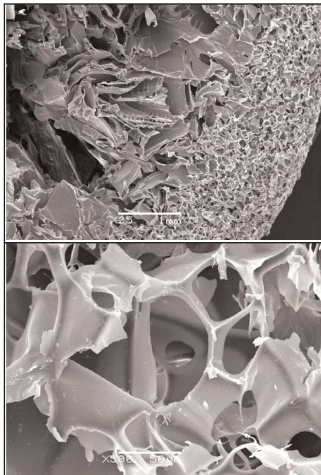
Figure 1. Scanning electron micrograph of the inner part of the supermacroporous poly(AAm-AGE) monolithic cryogel matrix.
