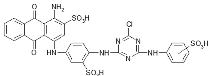
Figure 3. Chemical Structure of Cibacron Blue F3GA.
