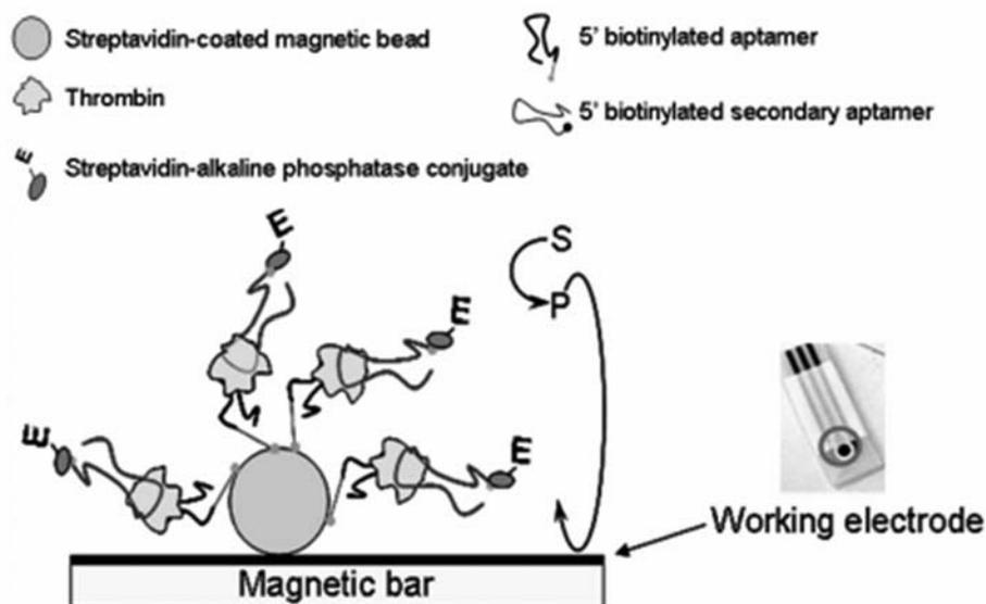
Figure 1. Scheme of the electrochemical sandwich assay coupled to magnetic beads.
