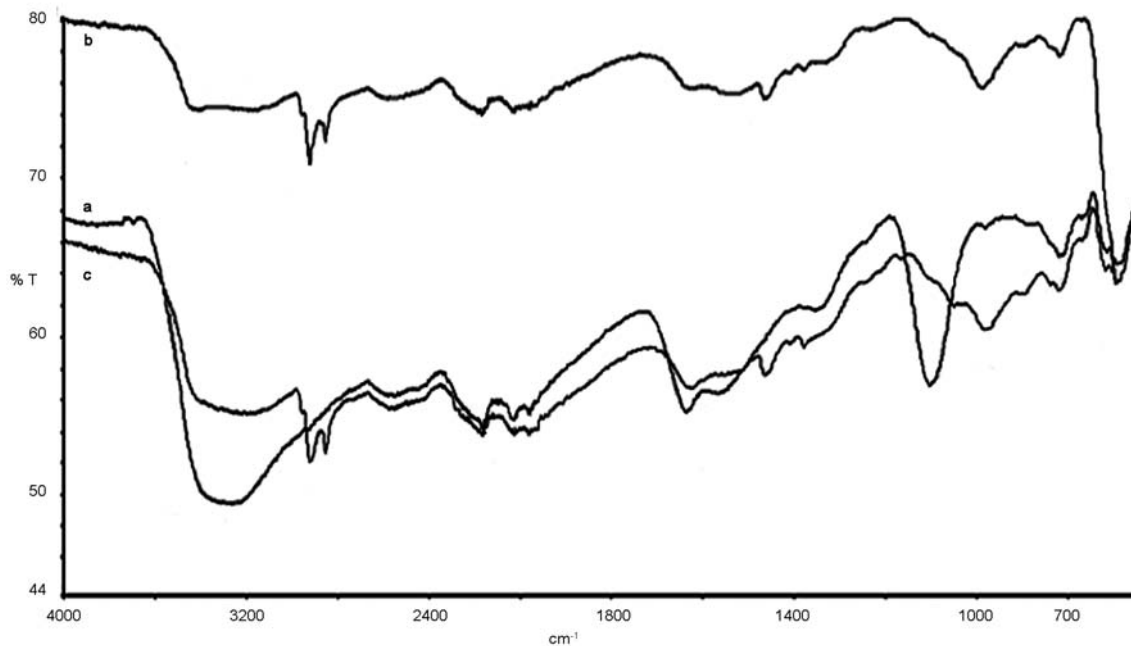
Figure 3. FTIR spectra of magnetite NPs (a), silanized NPs (b) and \text{Cu}^{2+} -attached silanized NPs (c).
