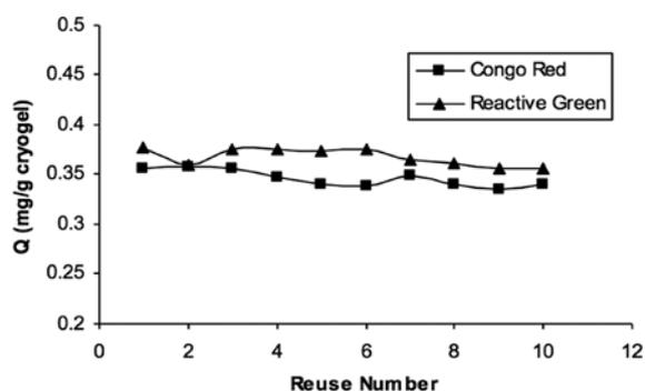
**Figure 9.** Reuseability of p(AAm-AGE)-CB-Fe<sup>3+</sup> cryogel for dye adsorption. c: 20ppm, pH: 6.0 for RG & CR, T: 25°C, flow rate: 0.3 mL/min, t: 8 min.
