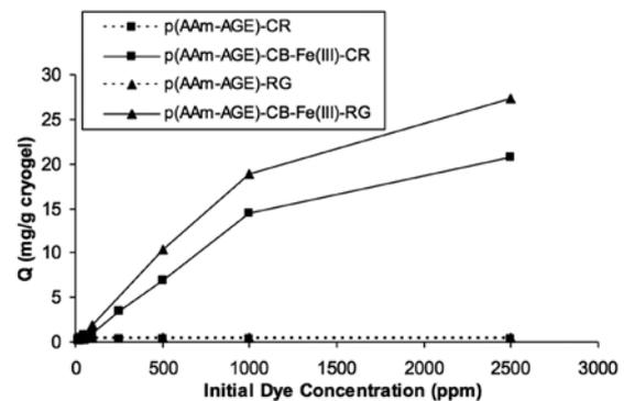
**Figure 6.** Effect of initial concentration on dye adsorption onto p(AAm-AGE)-CB-Fe<sup>3+</sup> cryogel. pH: 6.0, T: 25°C, flow rate: 0.3 mL/min, t: 8 min.
