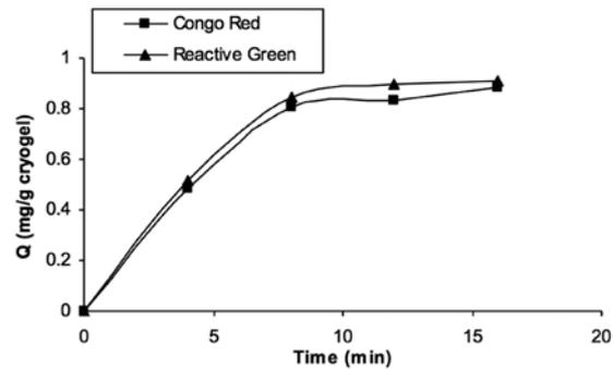
**Figure 4.** Effect of contact time on dye adsorption equilibrium onto p(AAm-AGE)-CB-Fe<sup>3+</sup> cryogel. c: 50 ppm, T: 25°C, flow rate: 0.3 mL/min.
