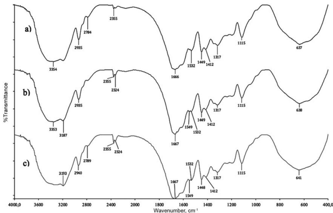
**Figure 3.** FTIR spectrum of p(AAm-AGE) (a), p(AAm-AGE)-CB (b) and p(AAm-AGE)-CB-Fe<sup>3+</sup> (c) cryogels.
