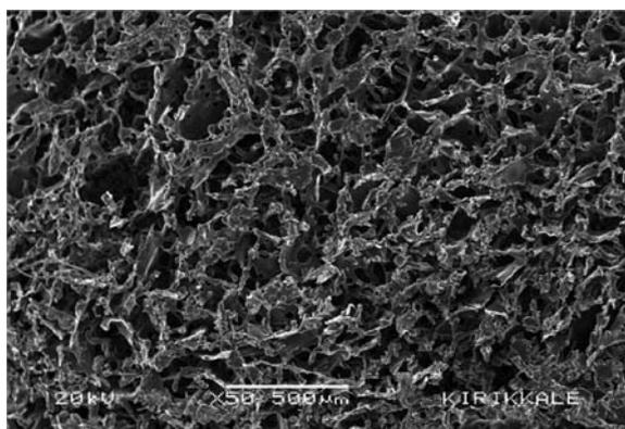
**Figure 1.** Scanning electron micrograph of the inner part of the p(AAm-AGE)-CB-Fe<sup>3+</sup> cryogel.
