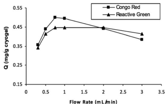
**Figure 8.** Effect of flow rate on dye adsorption onto p(AAm-AGE)-CB-Fe<sup>3+</sup> cryogel. c: 20 ppm, pH: 6.0, T: 25°C, t: 8 min.
