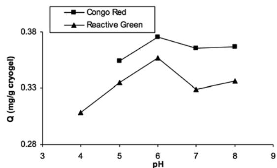
**Figure 5.** Effect of pH on dye adsorption onto p(AAm-AGE)-CB-Fe<sup>3+</sup> cryogel. c: 20 ppm t: 8 min, T: 25°C, flow rate: 0.3 mL/min.
