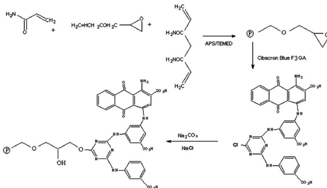
**Figure 2.** Schematic diagram for the production of p(AAm-AGE) cryogel and immobilization of dye molecules through the p(AAm-AGE) cryogel.
