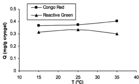
**Figure 7.** Effect of temperature on dye adsorption onto p(AAm-AGE)-CB-Fe<sup>3+</sup> cryogel. c: 20ppm, pH: 6.0, flow rate: 0.3mL/min, t: 8 min.**Table 2.** Freundlich constants for dye adsorption.
