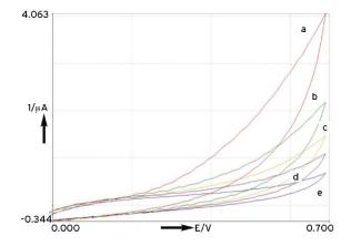
**Figure 1.** CVs of the mushroom (*Agaricus bisporus*) tissue homogenated based biosensor. (Phosphate buffer; pH 7.0, 50 mM, T: 30°C) (from a to e: baseline, 1.0, 2.5, 5.0, and 10.0 mM ethanol). The amount of homogenate, gelatine and percentage of glutaraldehyde were kept constant at 200.0 mg, 5.0 mg, and 2.5%, respectively. Scan rate is 25 mVs<sup>-1</sup> and potentials referred to Ag/AgCI reference electrode.
