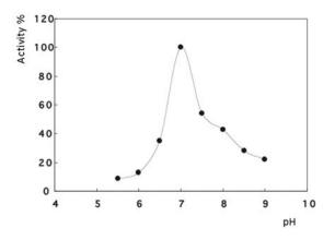
**Figure 2.** The effect of pH on the biosensor response (pH: 5-6, citrate buffer; pH: 6.5-8.0, phosphate buffer; pH: 8.5-9.0, glycine buffer. Concentration of all buffers is 50 mM). The amount of the mushroom tissue, the percentage of glutaraldehyde, gelatin amount and temperature were kept constant at 200 mg, 2.5%, 5 mg and 30°C, respectively.
