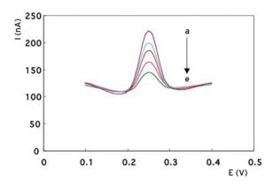
**Figure 3.** Differential pulse voltammograms obtained for different ethanol concentrations. (Phosphate buffer; pH 7.0, 50mM, T:  $30^{\circ}$ C) (from a to e: 1.0, 2.5, 5.0, 7.5 and 10.0 mM ethanol). The amount of homogenate, gelatine and percentage of glutaraldehyde were kept constant at 200.0 mg, 5.0 mg, and 2.5%, respectively.
