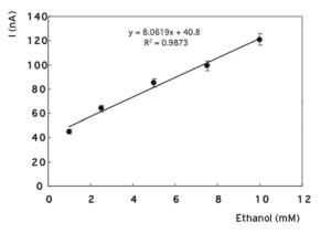
**Figure 4.** Calibration curve of the biosensor. (Phosphate buffer; pH 7.0, 50 mM). The amount of the mushroom tissue, the percentage of glutaraldehyde, gelatin amount and temperature were kept constant at 200 mg, 2.5%, 5 mg and 30°C, respectively.
