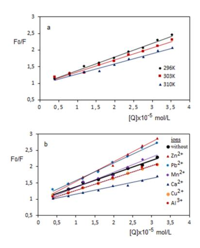
Figure 2. The effect of (a) temperature and (b) common metal ions on the Stern-Volmer plots of 7HC/insulin system.  $C_{insulin} = 5.0x10^{-6}$  M,  $C_{each ion} = 10x10^{-6}$  M at  $\lambda_{ex}/\lambda_{em} = 276/306$  nm.
