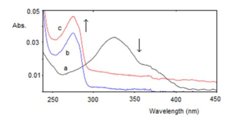
Figure 6. The absorption spectra of (a) 5.0x10<sup>-6</sup> M free 7HC, (b) 5.0x10<sup>-6</sup> M free insulin, (c) 5.0x10<sup>-6</sup> 7HC-5.0x10<sup>-6</sup> insulin system.
